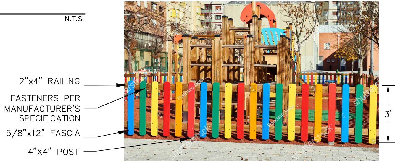
8 PLASTIC LUMBER FENCE DETAIL (ALTERNATE ITEM) N.T.S.
